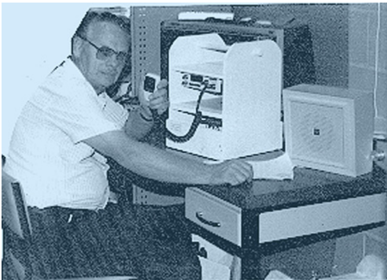
Figure 116.2 A simple school radio box with battery in lower section of cradle. The weight can be reduced by using lighter 12 V batteries. (Based on an original design by Kelvin Rodgers)
